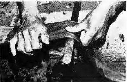
39. Shaping the wetted sides over a hot metal rod.
