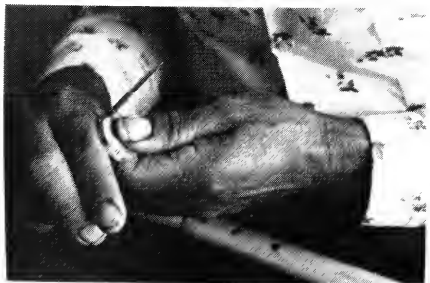
27. Cutting the diaphragm out of gourd.
