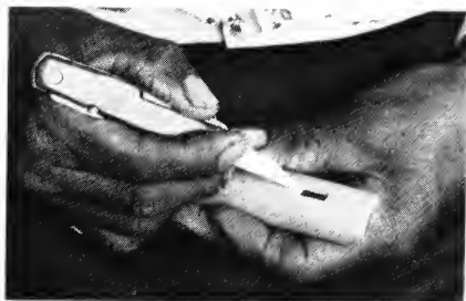
24. Cutting the blade-shaped edge into the hole of the tube.
